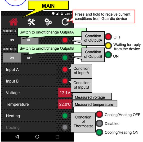
Please note that the temperature and thermostat features are available only if temperature sensor is connected to the device
